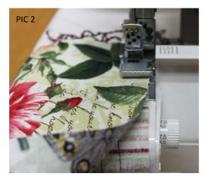
Convert your Baby Lock to a wide three thread flatlock, using the left needle with a decorative thread in the upper looper.
