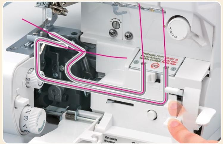
**JetAir™ with Tubular Loopers** allows you to thread in any order and avoid tangles and knots as threads are not exposed.
