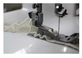
Remove the clear foot and replace with the standard/grooved foot. Convert the Ovation to a Chain Stitch using the C1 or C2 needle.
